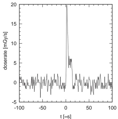
Fig. 4. Rate of absorbed dose in the BLM during the injection of beam in the proton ring.
