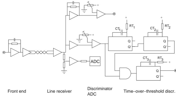
Fig. 2. Functional diagram of the electronics of the BLM showing the front-end electronics and the backend signal processing of a single channel.
