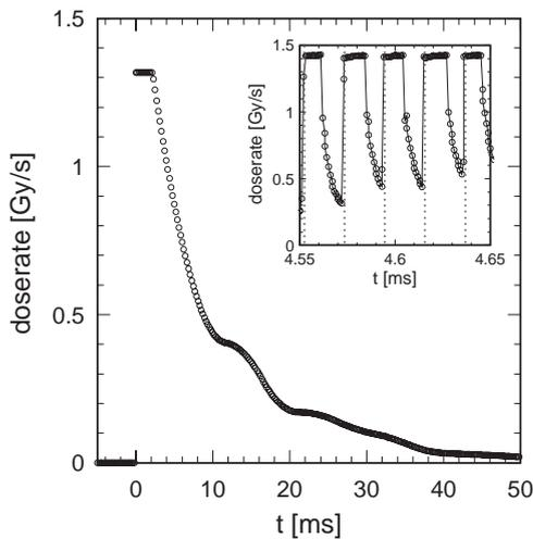
Fig. 3. Rate of absorbed dose in the BLM during the injection of beam in the HERA-positron ring. The data are smoothed, the insert shows the full (time) resolution. The vertical lines in the insert mark the consecutive revolutions of the same bunch.
