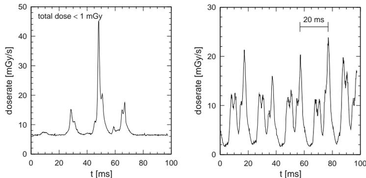
Fig. 8. Rate of absorbed dose in the BLM in periods associated with beam instabilities. Left-hand panel: transient which occurred during tuning of the beam for luminosity conditions. Right-hand panel: this condition lasted for several hours, the radiation is modulated with a 50 Hz noise.
