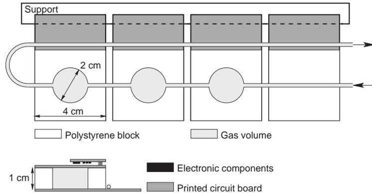
Fig. 1. Schematic diagram of the ionization chambers, showing the top view and the side view of the setup.
