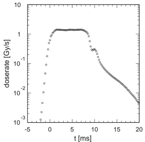
Fig. 6. Rate of absorbed dose in the BLM during an unexpected beam loss. The beam is lost in a few milliseconds, causing a high peak in the absorbed dose which decays with a time-constant of 3 ms.
