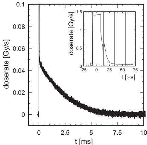
Fig. 5. Rate of absorbed dose in the BLM during an unexpected beam loss. The beam is lost almost completely in one revolution, causing a high peak in the absorbed dose (see inset), followed by a longer tail. The vertical lines in the inset mark the revolutions of the beam in the storage ring.
