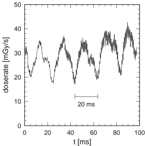
Fig. 7. Rate of absorbed dose in the BLM during an unexpected beam loss. The beam is lost in about 30 s, causing a high absorbed dose which is modulated with 50 Hz noise in this case.
