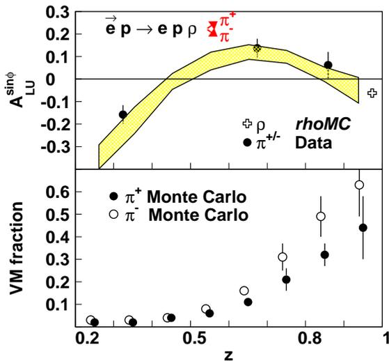
FIG. 4: Top panel: amplitude  $A_{LU}^{\sin\phi}$  for  $\pi^+$  mesons originating from  $\rho^0$  meson decays, obtained with Monte Carlo (band) and data (full circles). The open cross displays the asymmetry for the  $\rho^0$  itself (Monte Carlo). Bottom panel: the fraction of pions in the SIDIS sample originating from VM decays.
