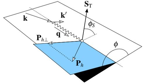
Fig. 1. The definition of the azimuthal angles  $\phi$  and  $\phi_S$  relative to the lepton scattering plane.
