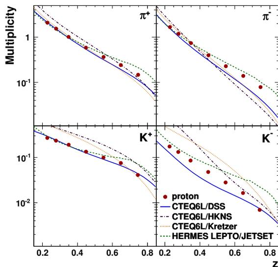
FIG. 2. Comparison of the vector-meson-corrected multiplicities measured on the proton for various hadrons with leading order calculations. Also shown are the values obtained from the HERMES Lund Monte Carlo. The statistical error bars on the experimental points are too small to be visible.
