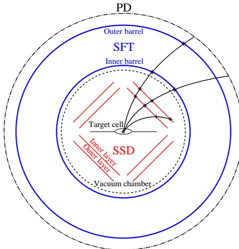
Figure 1: Schematic diagram of the HERMES recoil detector (cross-section view). The impinging electron beam is perpendicular to the paper plane. The cross section of the target cell is shown as ellipse. The curved lines denote reconstructed protons (tracks). The tracking layers are indicated, from inside to outside: Silicon Strip Detector (SSD, in diamond shape; one side of the diamond is about 10 cm long) and Scintillating Fiber Tracker (SFT, circles).
