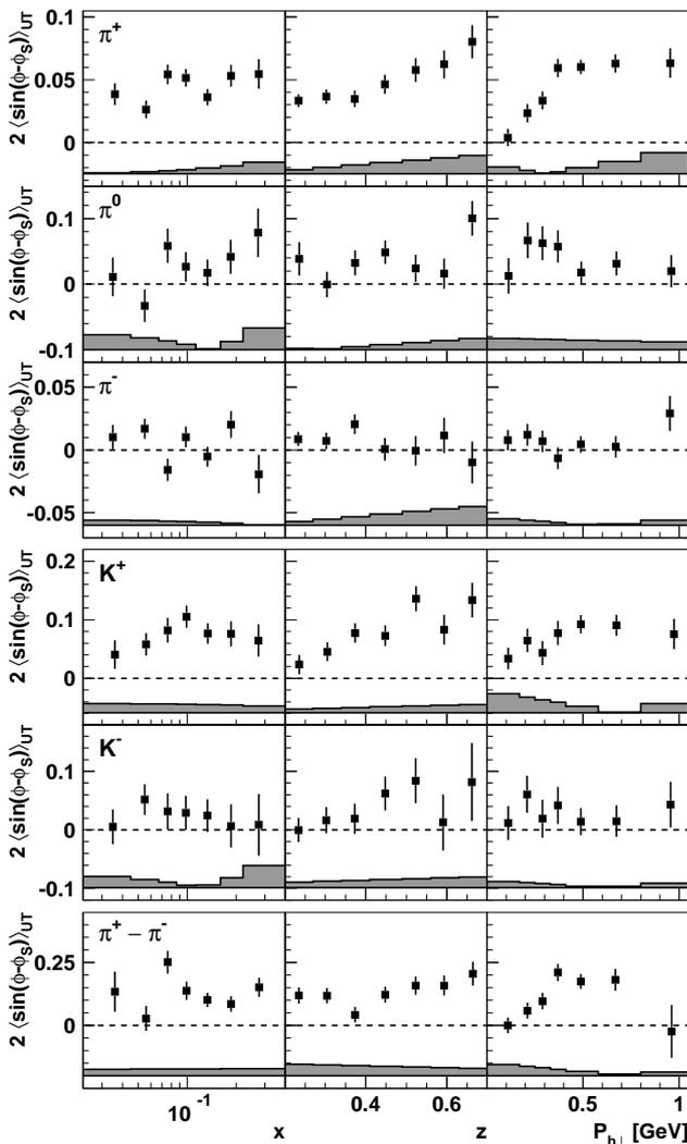
FIG. 1: Siivers amplitudes for pions, charged kaons, and the pion-difference asymmetry (as denoted in the panels) as functions of  $x$ ,  $z$ , or  $P_{h\perp}$ . The systematic uncertainty is given as a band at the bottom of each panel. In addition there is a 7.3% scale uncertainty from the target-polarization measurement.
